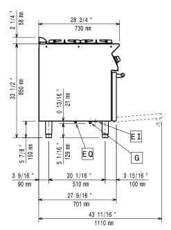
Electrical inlet (power) Gas connection
